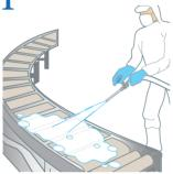
Use the foam cleaning system to spray the detergent solution onto the surface/object.
